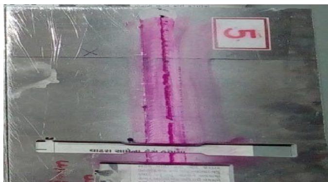
(B)Plate-5, Tool-1(800rpm, 40mm/min)
